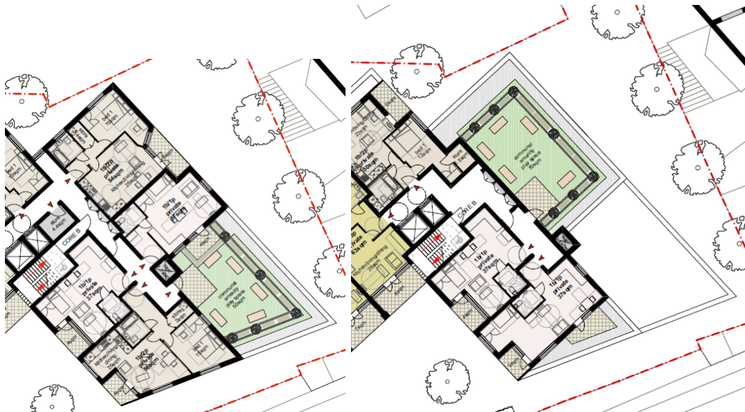
The 4 th and 5 th floor plans of the eastern block showing the roof top amenity areas.
